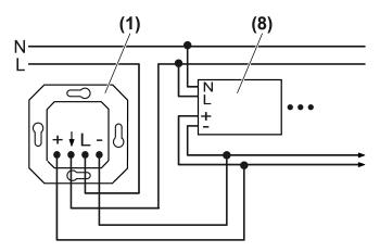
Image 2: Connection diagram - Potentiometer switches the lamp operating devices directly
