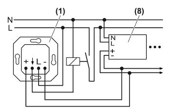
Image 3: Connection diagram - Potentiometer and contactor for switching the lamp operating devices
