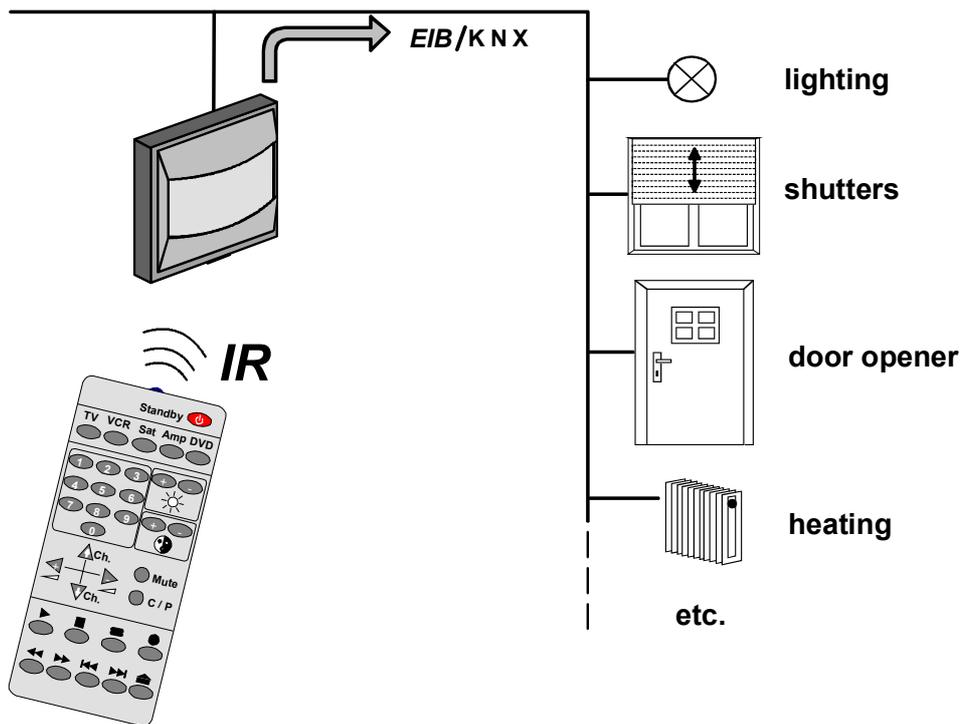
Fig. 2: Controlling the existing EIB/KNX installation with an IR transmitter
