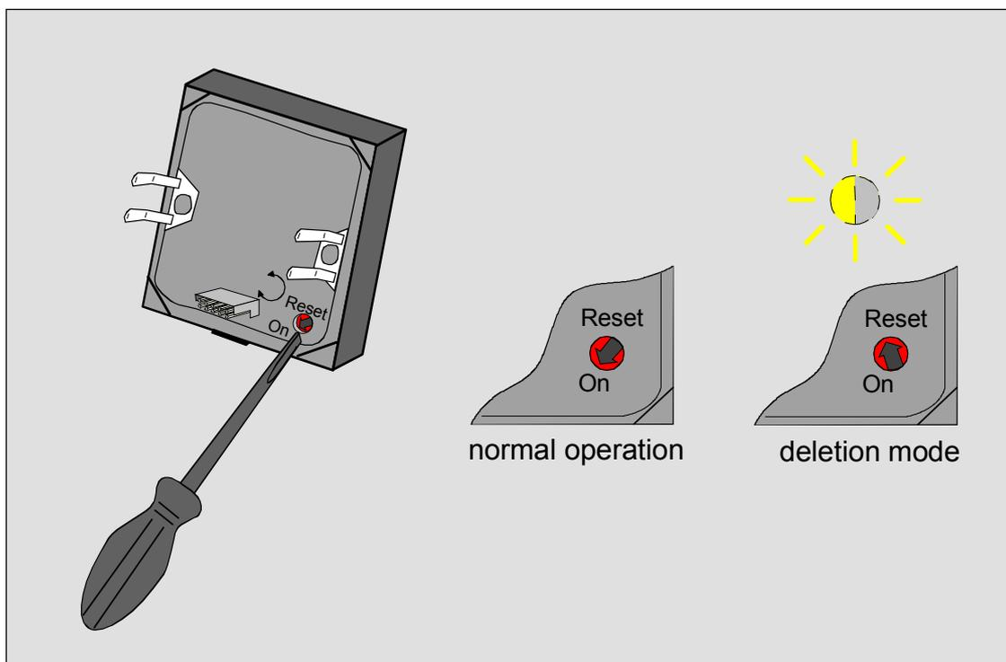
Fig. 12: Potentiometer at the back for activation or deactivation of deletion mode
