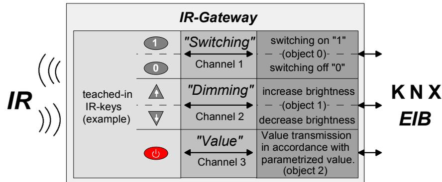
Fig. 7: Example of conversion from EIB/KNX bus telegrams into IR signals and vice versa
