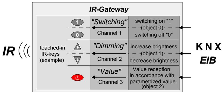
Fig. 5: Example for the conversion of EIB/KNX bus telegrams received into IR signals
