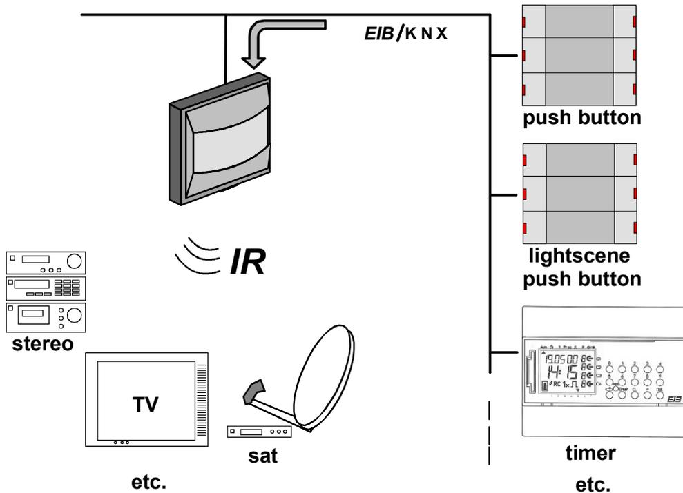
Fig. 4: Controlling existing IR components with sensors of the EIB/KNX installation
