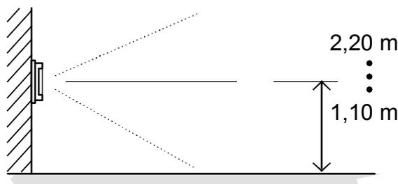
The gateway can be installed at hand level (1.10 m), but also at a height of 2.20 m.
