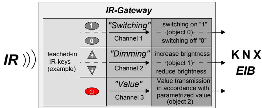
Fig. 3: Example of IR signals received controlling EIB/KNX bus datapoints
