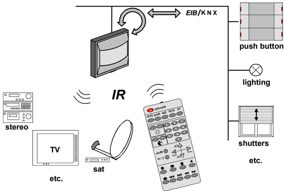
Fig. 10: Activation of different IR signals stored in the IR-Gateway from an IR remote control
