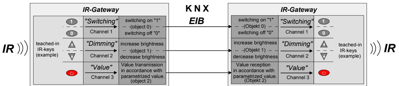
Fig. 9: Example of conversion of IR signals by two Gateways
