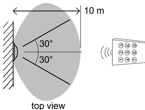
The range (approx. 10 m) is optimal within an angle  $30^\circ$  (from the median line). Even greater distances and angles can be achieved when transmitter and receiver are arranged in a straight line. The same applies, if the IR light can be reflected from walls or pieces of furniture in the room.
