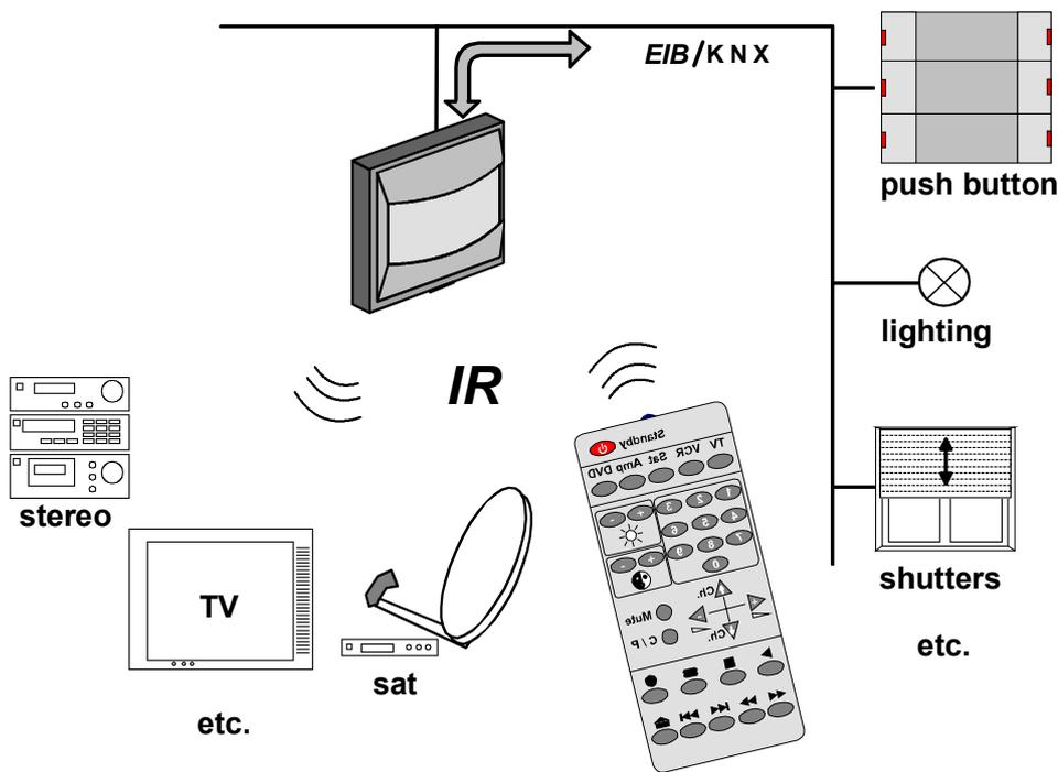
Fig. 6: Bidirectional control of existing IR components and of the EIB/KNX installation
