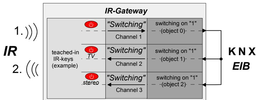
Fig. 11: Conversion of an IR signal into one or several other previously programmed signals
