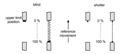
A reference movement is the time needed for a movement into the upper limit stop position prolonged by 20 % and additionally by the parameterized moving time extension. The moving time can be adjusted separately for each output channel. A reference movement cannot be retriggered.
