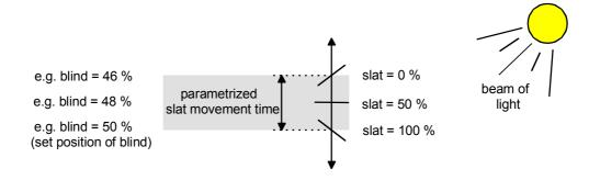
This example shows that slat angle changes result in a new blind position which is also followed up in the positioning objects. If the actuator receives in this case a 'new' blind position of e.g. 47 %, the actuator does not induce a movement, as the computed moving time falls into the parameterized slat moving time and thus coincides with the slat movement. A change of the blind position to 55 % in this example induces a blind movement as the change lies beyond the slat movement (0 to 100 %).
