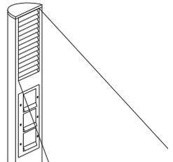
5. Set the profile cover in place and fasten it with both cover screws.
