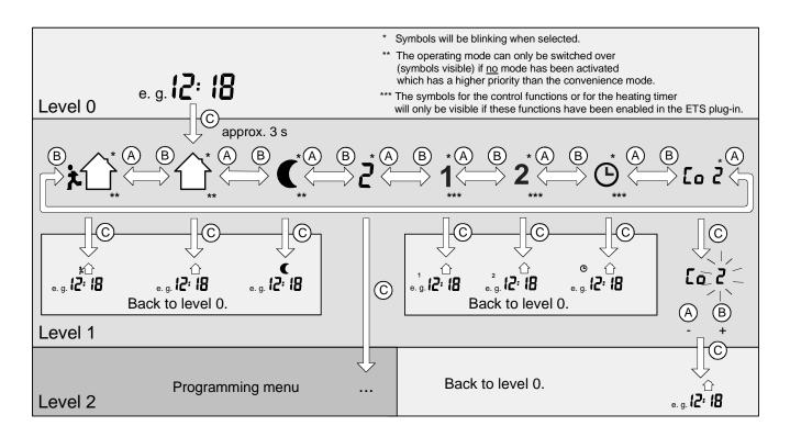
If you have set the "access to operator levels" to "first operator level" or "all operator levels" you can actuate the middle of rocker 1 ( $^{\odot}$ ) for at least 3 s to change to operator level 1. At this position, you can select the controller operating mode and activate or deactivate the heating timer or the control function(s). You can also adjust the display contrast.
