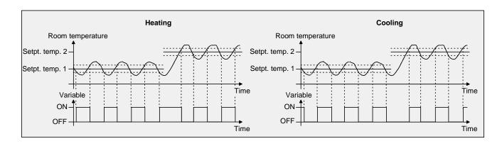
An additional heating or cooling stage as 2-point control works in the same way as the 2-point control of the basic stage, with the exception that the setpoint and the hysteresis values will shift, taking account of the parameterized difference between the basic and additional stages.
