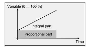
An additional heating or cooling stage as PI control works in the same way as the PI control of the basic stage, with the exception that the setpoint will shift, taking account of the parameterized difference between the basic and additional stages.
