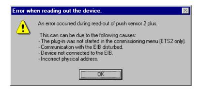
Fig 3: General communication error during a reconstruction
