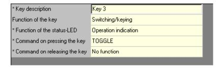
Fig. 1: Example for global parameters marked by the asterisk
