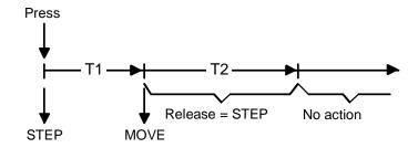
When the key is being pressed a STEP message will be sent and start time T1 ("time between short-time and long-time mode") started. If you release the key within time T1 no further telegram will be sent. This STEP serves for stopping an ongoing continuous run.
