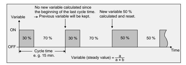
For a variable of 0 % (permanently OFF) or of 100 % (permanently ON), a variable telegram corresponding to the variable value ("0" or "1") will always be sent after a cycle time has elapsed. 'Clipping' (refer to "continuous PI control") will also be active for this type of control.
