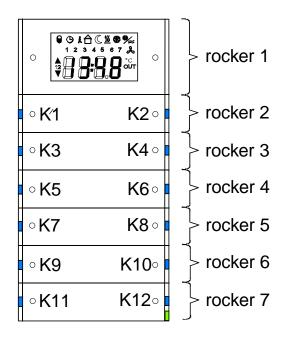
Depending on the application (2fold, 3fold or 6fold) inserted into the ETS project, the required number of rockers or keys, respectively, will be created automatically in the ETS plug-in.
