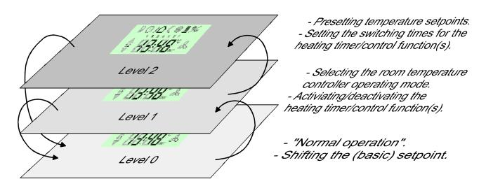
The "access to operator levels" parameter in the "push sensor 2 plus" parameter branch specifies which levels you can activate by local operation.
