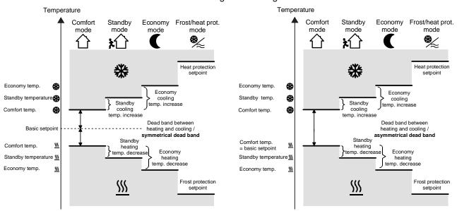
Temperature Control with Additional Stage by the "Heating and Cooling" Example with Symmetrical Dead Band...
