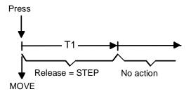
When a key of the rocker is being pressed a MOVE signal will be sent, and start time T1 ("lamella adjustment time") will be started. If you then release the key within time T1 the push sensor will send a STEP telegram. This function is used for lamella adjustment. T1 should correspond to a 180° lamella rotation.
