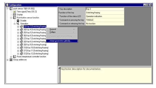
Fig. 3: Activating global adaptation of parameters in the selected branch by means of the context menu
