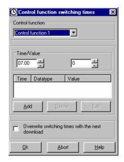
After you have set the switching time and the control command, you can click on the "add" button to create the switching program. You can create the maximum of the two switching programs per control function from the program list in the middle of the window. If you highlight a program in the list and click on the "edit" button you can edit this program. Highlighting a program and clicking on the "delete" button will delete the program and remove it from the list.
