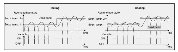
An additional heating or cooling stage as 2-point control works in the same way as the 2-point control of the basic stage, with the exception that the setpoint and the hysteresis values will shift, taking account of the parameterized difference between the basic and additional stages.
