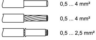
Figure 5: Clampable cable cross-sections
