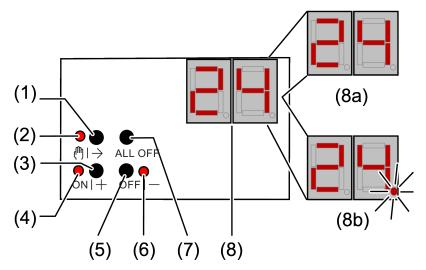
Figure 1: DALI Gateway control panel, 1fold
