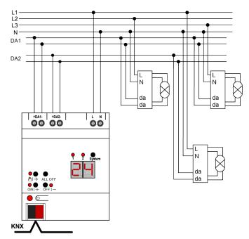
Figure 3: DALI gateway connection example, 2fold
