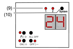
Figure 2: DALI Gateway control panel, 2fold
