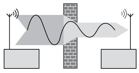
Figure 2: Reduced range due to structural obstacles
