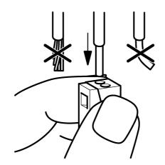
Figure 7: Connection of the single-stranded cable
