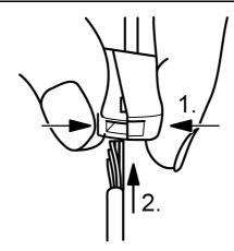
Figure 6: Connection of the fine-wire cable
