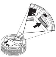
When locking the smoke alarm device into the mounting plate/230 V base, the smoke alarm device is activated automatically. Alternatively, the activation button for the function test can also be held manually (the power supply of the smoke alarm device is activated automatically. Initialisation phase 30 s).
