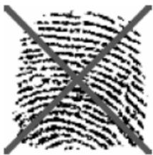
The sensor only then scans the fingerprint in the upper section of the finger pad, far above the fingerprint swirl. Here are significantly less curved skin lines, meaning that the system cannot recognise sufficient significant features.
